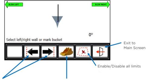
Set a left or right virtual wall which will be parallel with the tracks or wheels of the machine.
