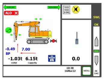
If the Bucket Pin goes below the target level, then the down arrow will be red (see adjacent picture) and the Boom Down motion will be cut to prevent digging down any further.
