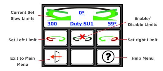
To set slew limits, slew the machine left to required position and press the "Set Left Limit" button.
