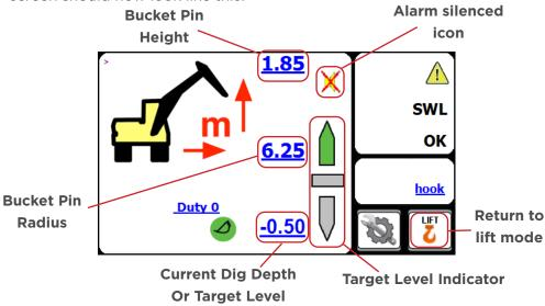
To exit Dig Mode and return to Lifting Mode, press on the "Return to Lift Mode" button, shown above.
