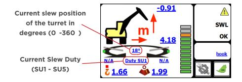
Typically, eight slew "duties" are available. The duties are named SU1 - SU5, with each duty having it's own calibrated "tip" point for the machine.
