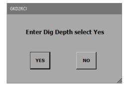
Pressing "NO" will allow the operator to use the position entry mode.
