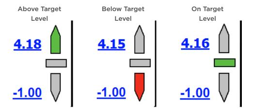
**NOTE** - The depth indication is measured to the load point. The orientation of the bucket will affect the accuracy of the indicator. Moving the machine from one level to another will change the depth of a trench. Whenever the machine is moved it is recommended that the depth is reset by placing the bucket on the level previously dug and reset the depth by pressing dig mode, "**NO**" and "**YES**" to make the new bucket position to datum.
