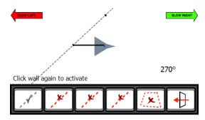
The "**Set Virtual Wall 1**" button will now be greyed out. Pressing on this button will activate the virtual wall and the button will change to indicate that the virtual wall is not active.
