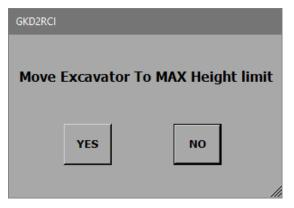
Press "YES" when the machine is in the correct position.
