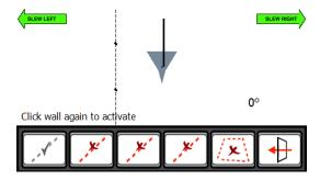
The "Set Virtual Wall 1" button will now be greyed out. Pressing on this button will activate the virtual wall and the button will change to indicate that the virtual wall is not active.
