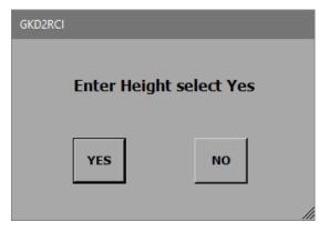
Pressing "NO" will allow the height to be set by moving the machine to the maximum height.
