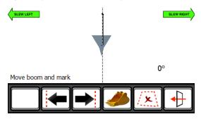
Slew the machine to move the bucket to the second position. As the machine moves, you will see the screen update and create a virtual wall between the first point and where the bucket is.
